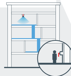
Maintenance shuts main valve
