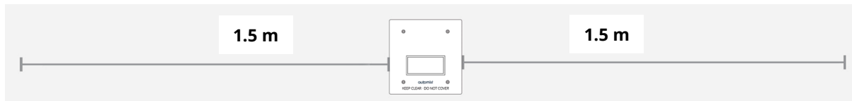
Figure 13: Keep 1.5m horizontal clearance around the spray head
