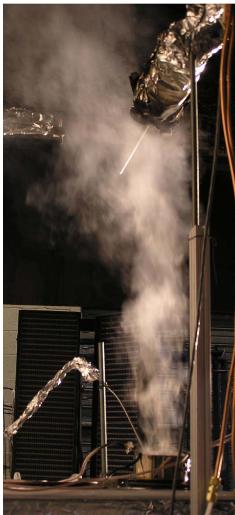
Figure 3-4. Plume of cooking oil vapor above pan before ignition during Test 2.
