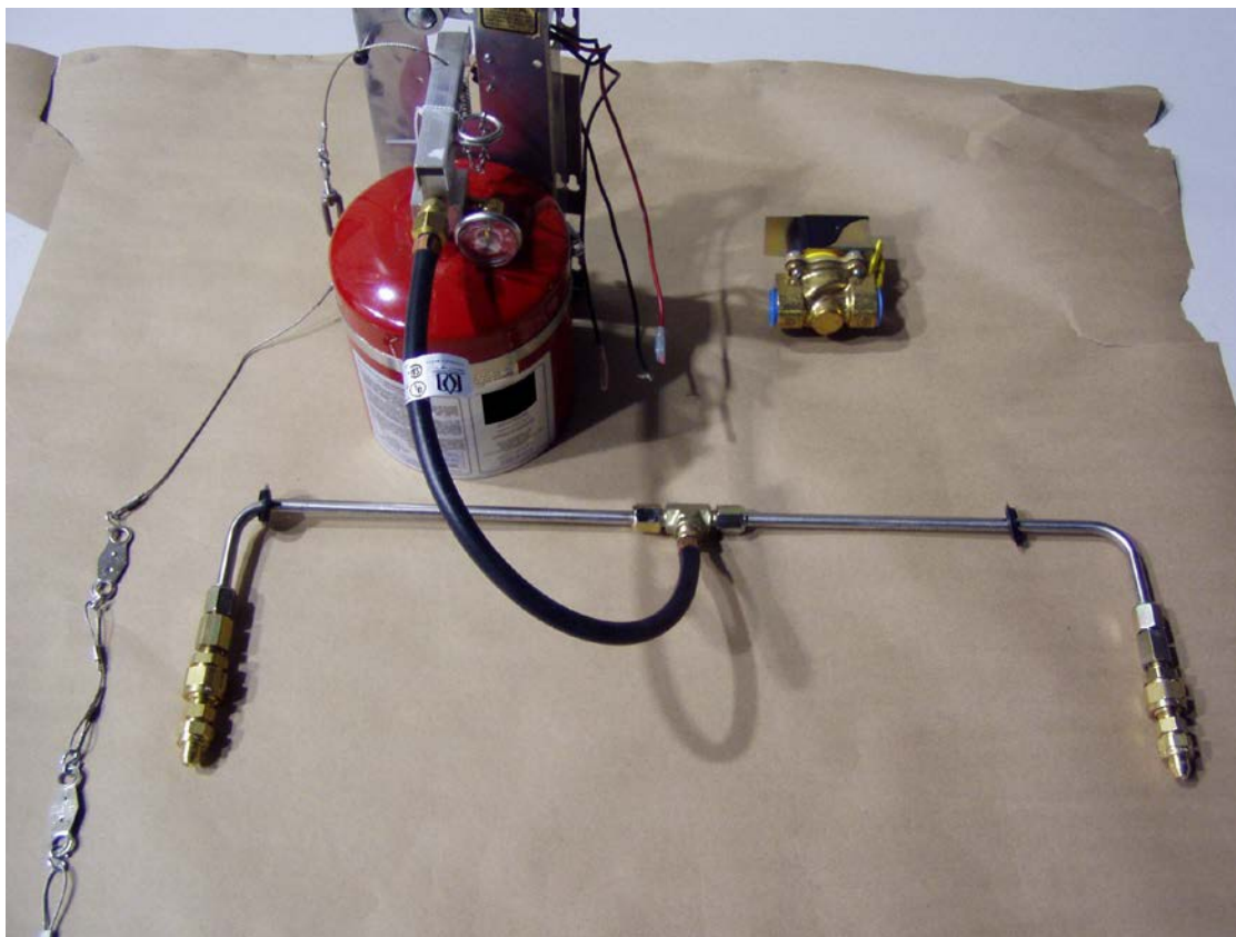
Figure 2-1. Components of an automatic, self-contained, wet chemical system (AWC1) including the automatic gas stovetop shutoff valve, which was not used in these experiments.
