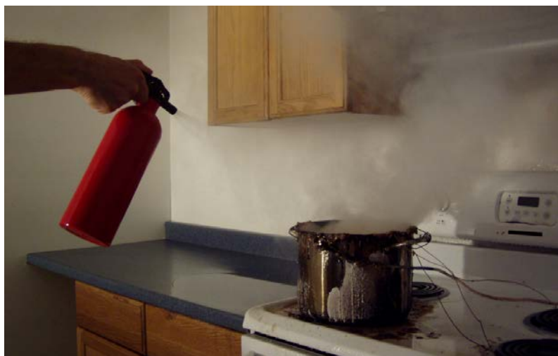
Figure 2-10. Discharge of manual wet chemical extinguisher.
