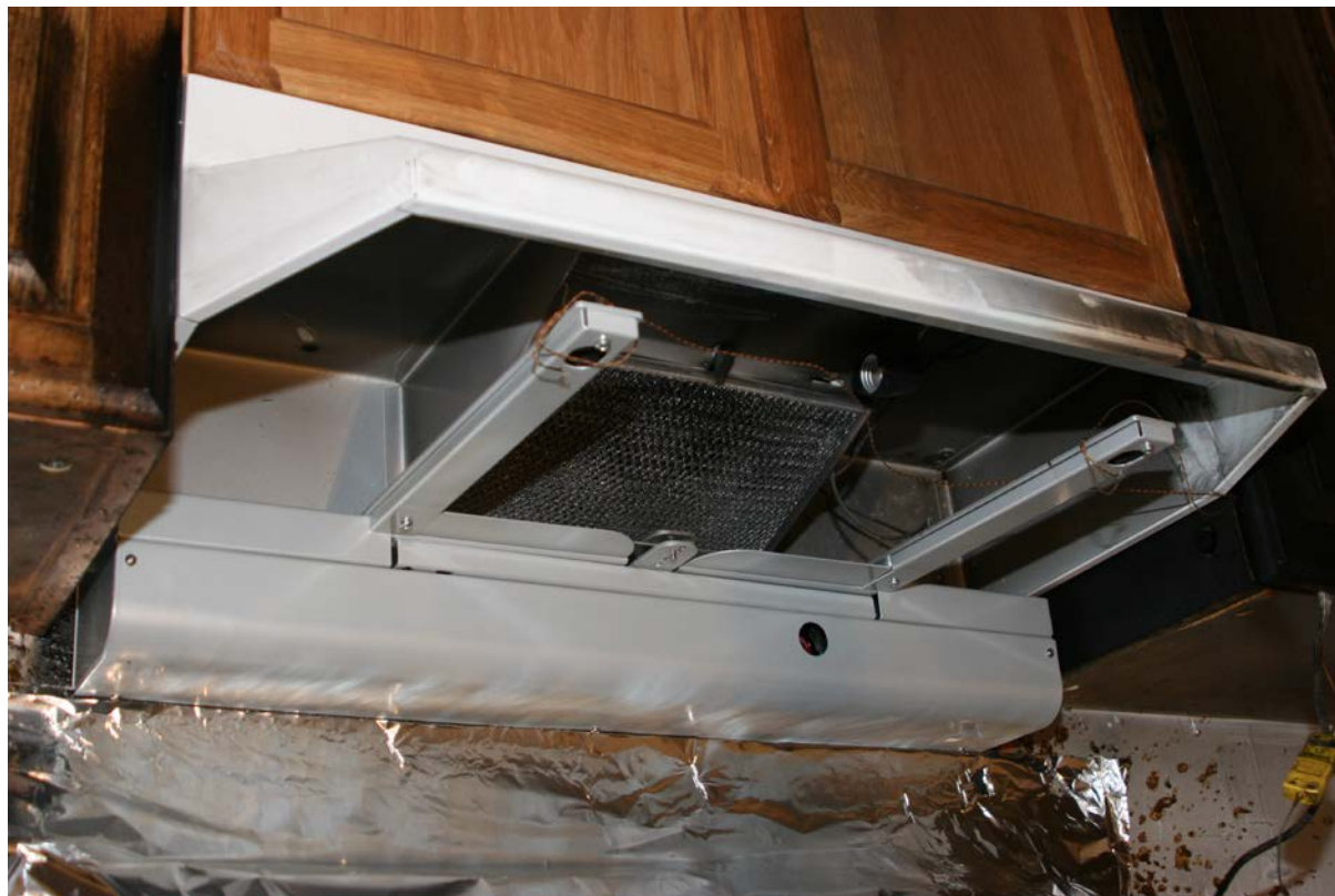
Figure 2-4. A wall-mounted, wet chemical system with arms containing heat sensitive bulb used to trigger agent deployment. Thermocouples mounted on the arms were not an intrinsic part of the device.
