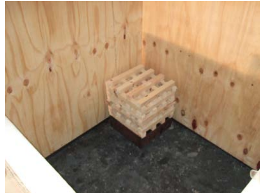
Photographs of ignition and fuel package before a test
