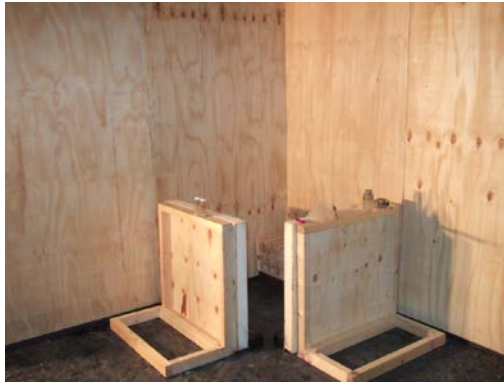
Photographs of ignition and fuel package before a test
