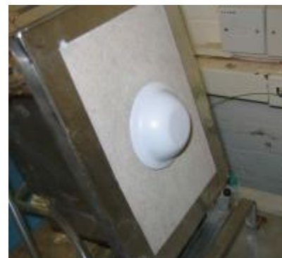
Concealed head with concealer plate prior to test
