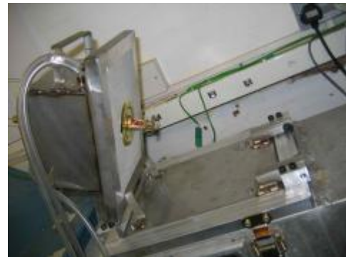
Pendent sprinkler prior to plunge test
