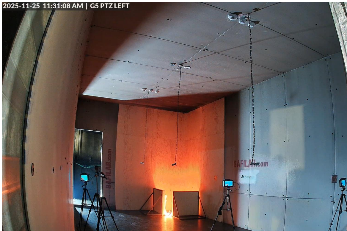
Photo B.1. Test no. 251125-2, corner test, 3.5m – before water mist system activation.
