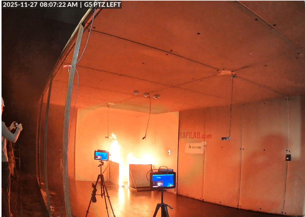
Photo B.7. Test no. 251127-1, corner test – open room, 2.5m – after water mist system activation.
