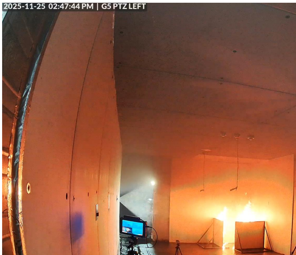
Photo B.4. Test no. 251125-4, corner test, 2.5m – after water mist system activation.
