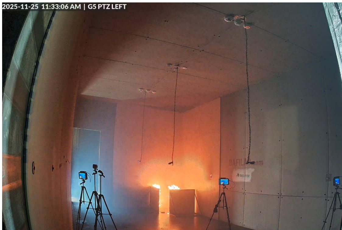
Photo B.2. Test no. 251125-2, corner test, 3.5m – after water mist system activation.
