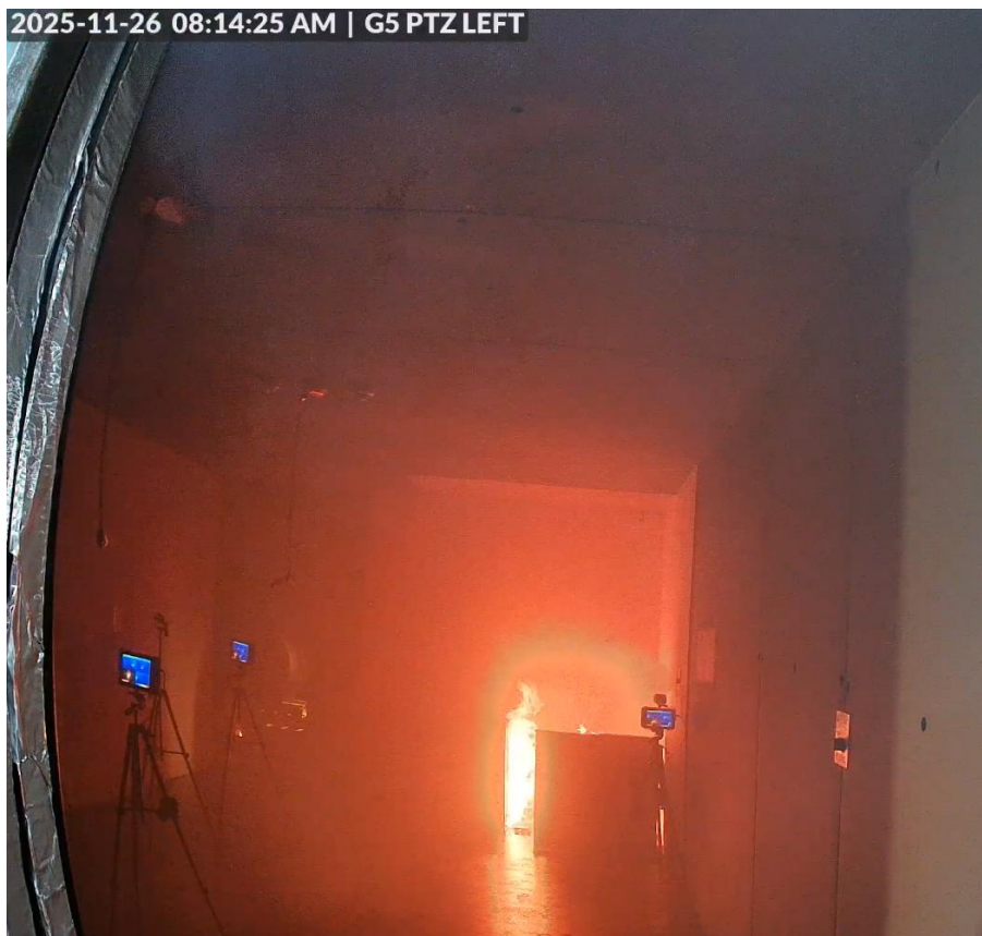
Photo B.6. Test no. 251126-1, corner fan test, 2.5m – after water mist system activation.
