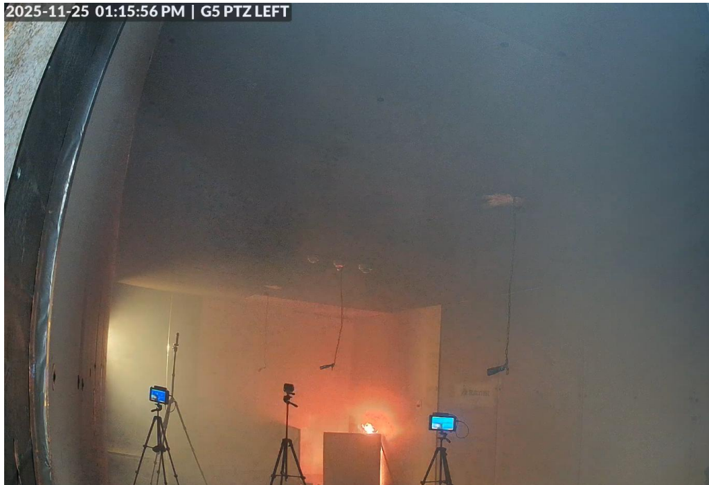
Photo B.3. Test no. 251125-3, corner test, 2.5m – after water mist system activation.
