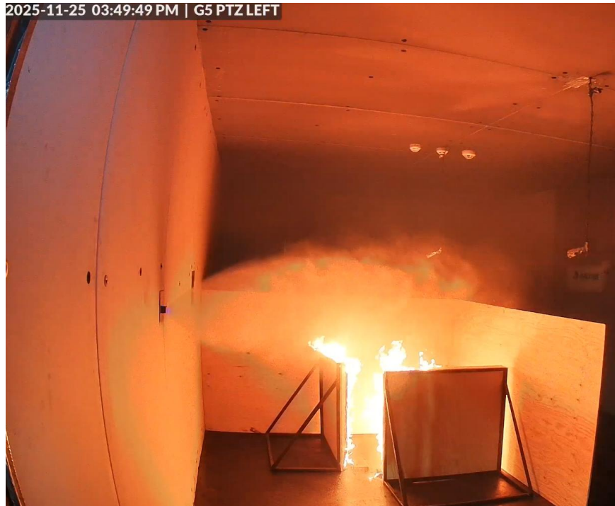
Photo B.5. Test no. 251125-5, B2 test, 2.5m – after water mist system activation.
