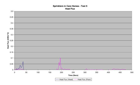
Note: No heat release rate measurements were carried out in Test 5.
