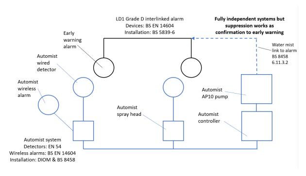
Figure 46: Watermist system linked to alarm system to provide fire confirmation as per BS 8458 6.11.3.2
