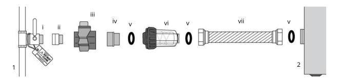
Figure 2: Automist Smartscan Hydra System Water Supply Components
