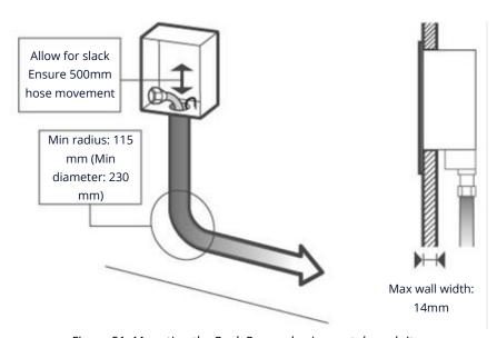
Figure 51: Mounting the Back Box and using metal conduits
