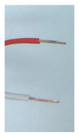
Figure 65: Cable (Firetuf 387FTD103) silicone insulation.
