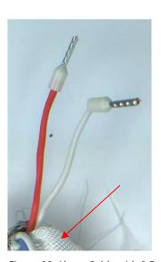
Figure 66: Alarm Cable with 0.5mm2 ferrule
