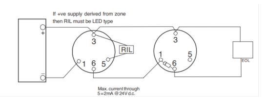
Figure 55: Wiring for Plumis DT02 wired detector
