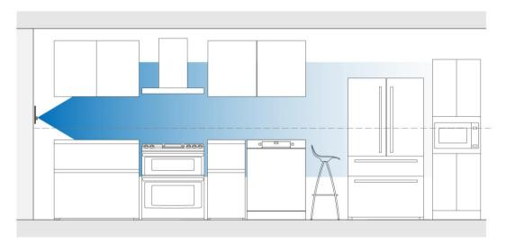
Figure 12: Diagram of the spray head height in relation to typical kitchen furniture
