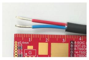
Figure 63: Cable (39200502H-E00) 30mm jacket crimped removed, 10mm insulation removed.
