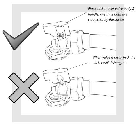
Figure 76: Water valve tamper label
