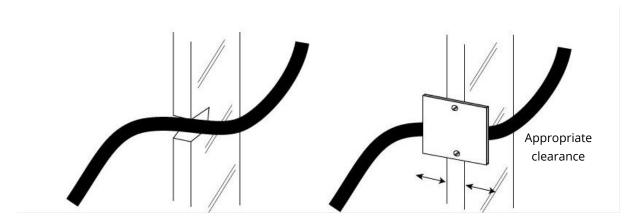
Figure 52: Example of mechanical protection within a joist
