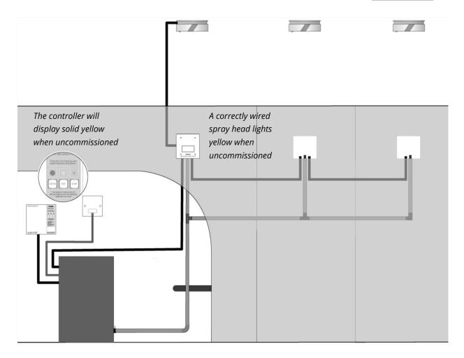
Figure 75: Testing the initial setup
