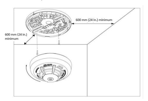
Figure 58: Mounting the detector
