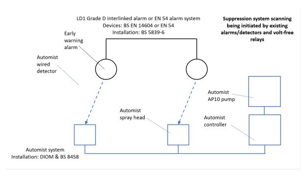
Figure 43: Volt-free detector relay bases used to initiate the scanning of Automist
