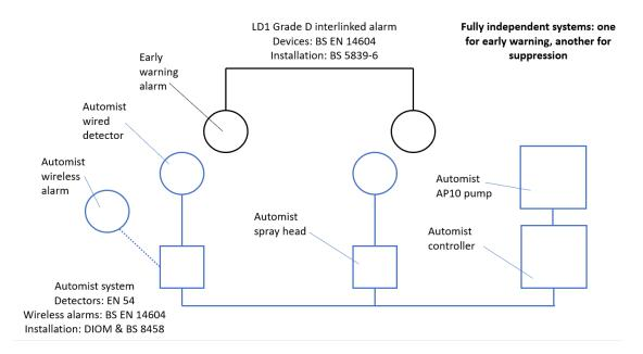
Figure 42: Early warning and suppression system independent systems
