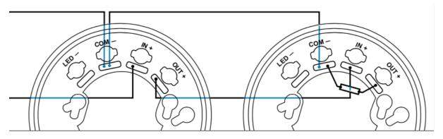
Figure 57: Mounting the resistor on wired Apollo detectors in chain
