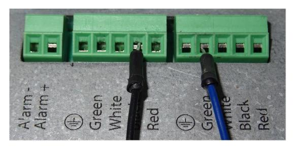
Figure 70: Connections on the spray head
