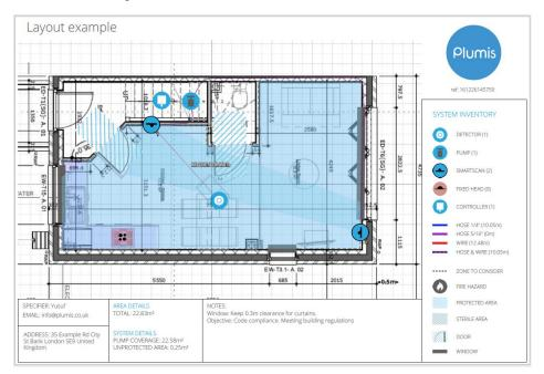
Figure 4: Automist Layout drawing
