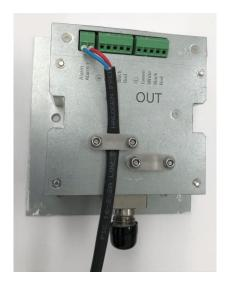
Figure 72: Alarm cable in spray head alarm connector
