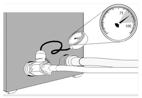
Figure 88: The pressure gauge during commissioning.
