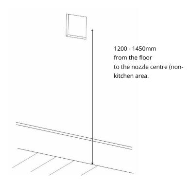
Figure 9: Automist Smartscan Hydra spray head mounting hole (non-kitchen area)
