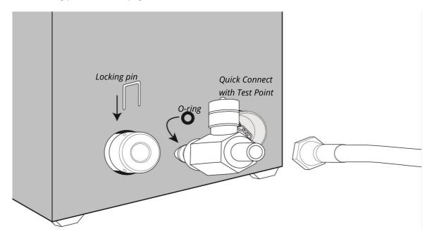
Figure 77: Connecting the Quick Test Point
