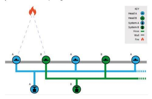
Figure 36: Installing two Automist systems in parallel
