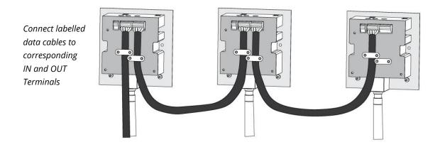
Figure 71: Spray head daisy chain connection
