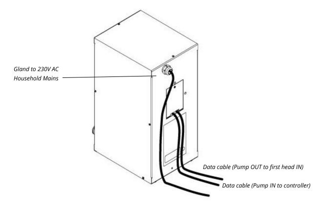
Figure 74: The pump front panel
