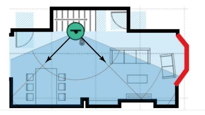
Figure 26: Example of a good spray head location with good line of site to the living room fire risks
