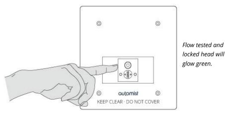
Figure 89: Remove flow test kit and gently tap to close head and lock
