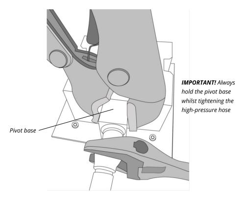
Figure 73: Spray head water path connection
