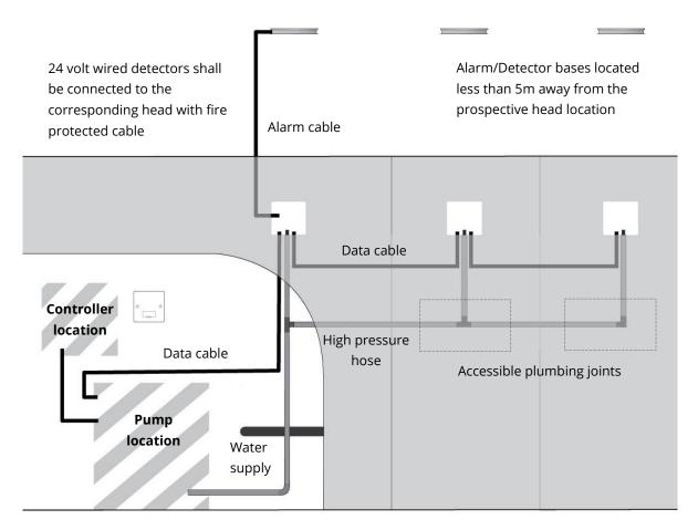
Figure 50: First Fix Setup
