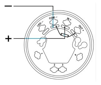
Figure 56: Mounting the resistor on wired Apollo detector
