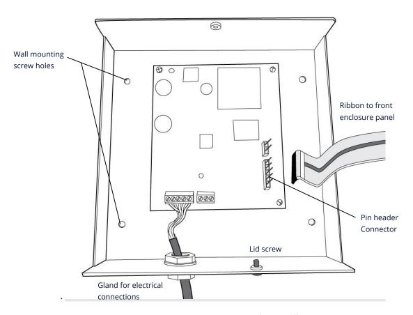
Figure 60: Connecting the controller
