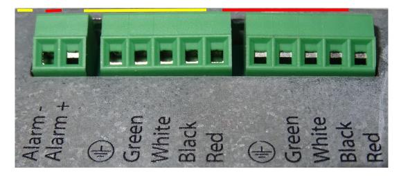
Figure 69: Screw terminals on the spray head
