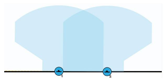
Figure 34: Utilising one spray head proximity to another
