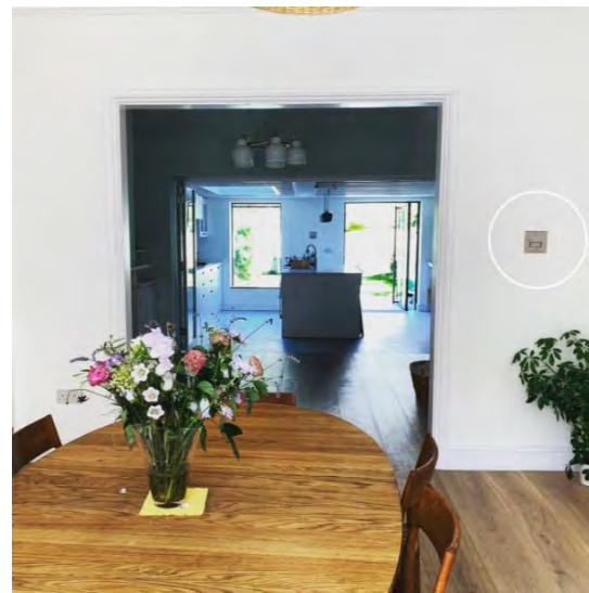
Figure 30: Preferred position alongside a door
