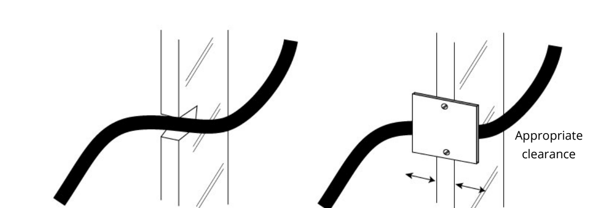
Figure 52: Example of mechanical protection within a joist
