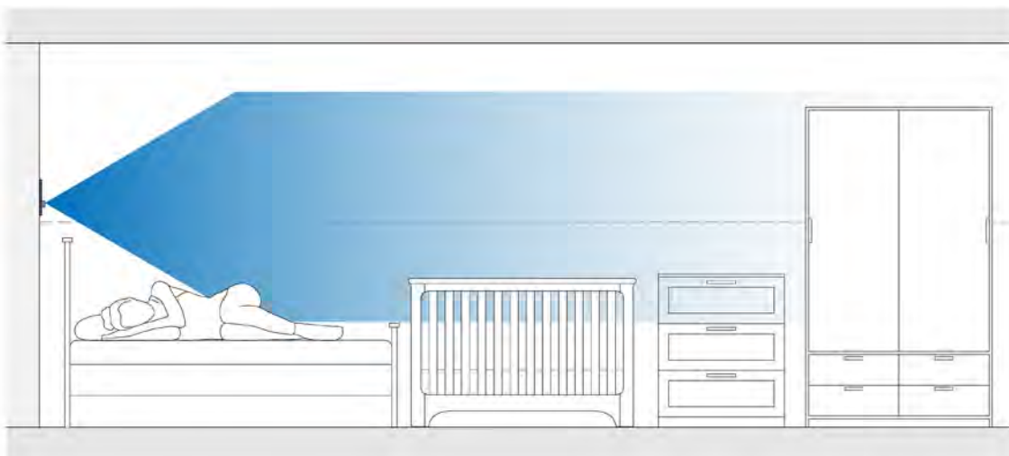
Figure 13: Drawing of the spray head height in relation to typical bedroom furniture
