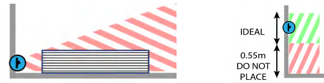
Figure 35: Preferred position >0.55m from adjacent wall
