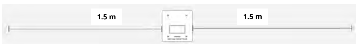
Figure 27: Keep 1.5m horizontal clearance around the spray head
