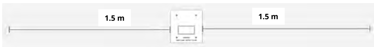
Figure 97: Keep clear of obstructions zone (min. 1.5m)
