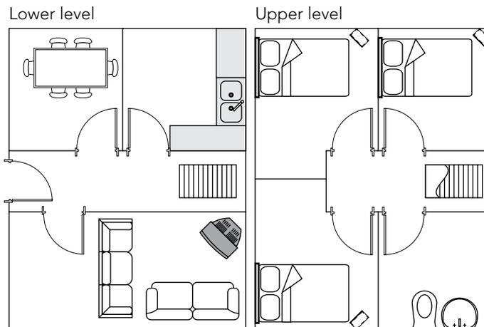
**Figure 20** Conventional AD B compliant two-storey flat.
