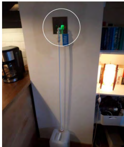
Figure 23: Preferred position in front of a nib (at least 0.3m deep and 0.25 - 0.6m wide)
