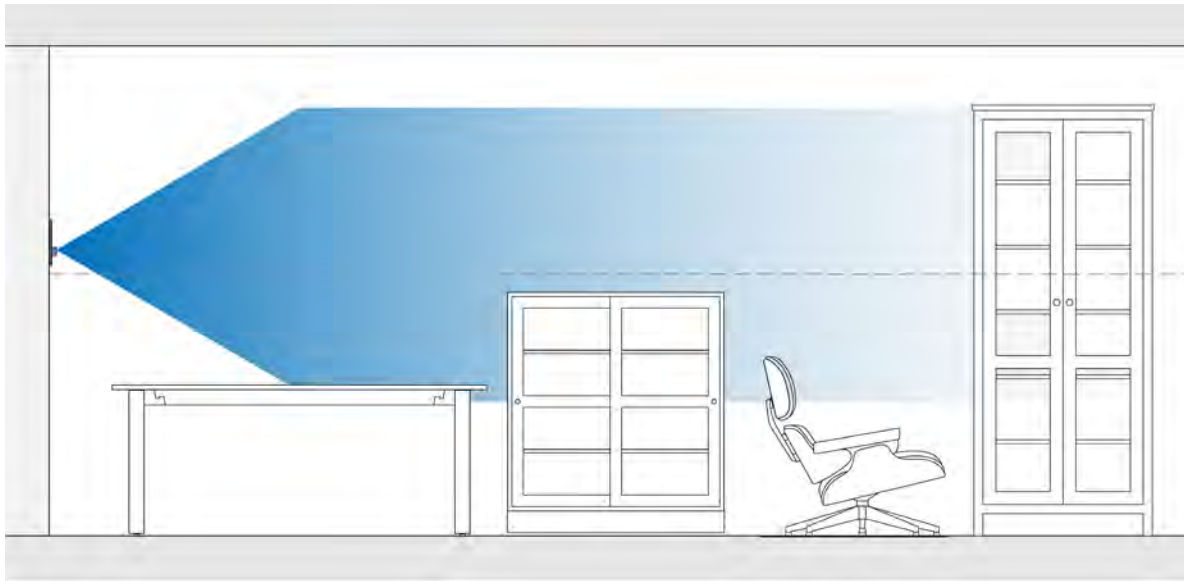
Figure 14: Drawing of the spray head height in relation to typical living room furniture
