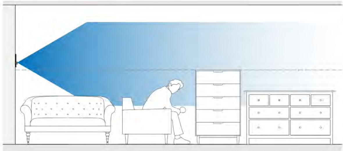
Figure 11: Diagram of the spray head height in relation to typical living room furniture
